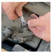
Connect the red wire connector to the terminal of the second battery. There is a voltage of 24V in the installation of the truck, which comes from two interconnected 12-volt batteries. It is important that the device is connected to the negative terminal of the first battery and the positive terminal of the second battery.
